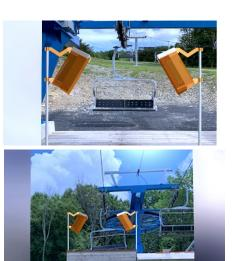
necessary amount of UV energy to deactivate any viruses or bacteria on the chair and safety bar. The one challenge is to make sure the UV is not visible to avoid possible eye exposure. This is being addressed with banners that are lifted on both sides of the chair path with sufficient room for clearance.
